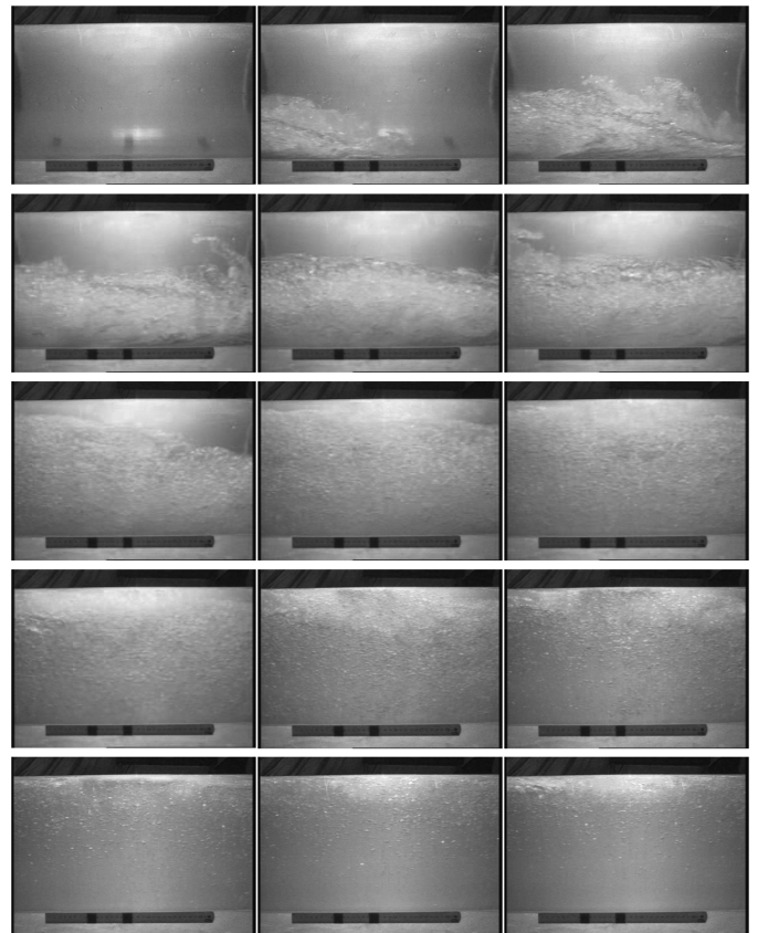
Fig. 10. Water front evolution at x = 249.5 m in the filling process (snapshots by video camera with a 0.04-s time interval starting at t = 50 s)
